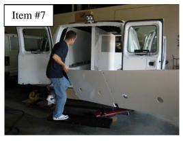
Carefully place **Driver-side Ceiling** section into vehicle.
